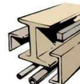
rods, angles, beams, channels
